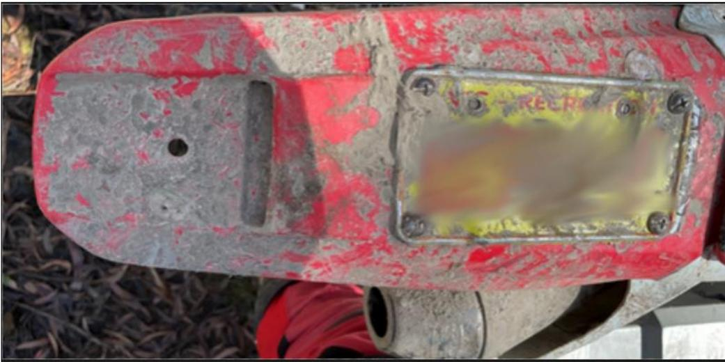
The images below show an acceptable rear guard with extension but an **unacceptable** mounting location of the number plate
