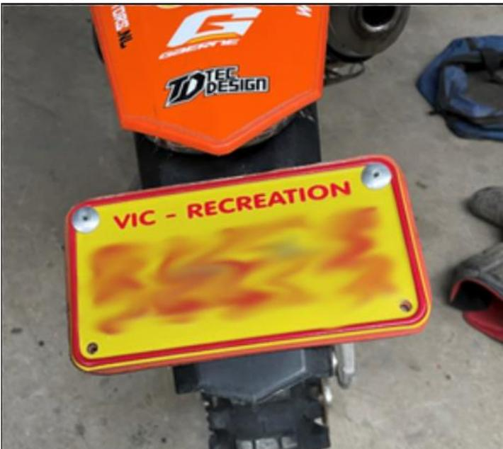
The images below show an acceptable rear guard with extension and accepted mounting of the number plate.
