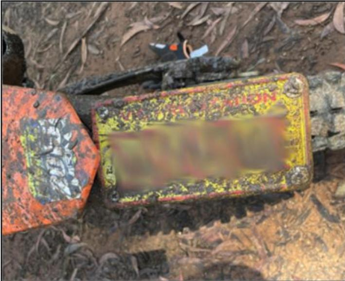
The images below show an **unacceptable** rear guard with no extension and **unacceptable** mounting location of the number plate.
